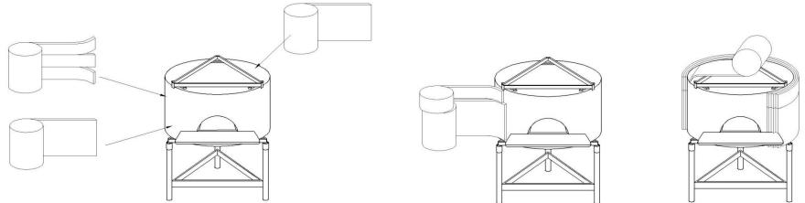
Wrap the oven with the insulating blanket. Put it all around 3 times and also on the top of the oven.
