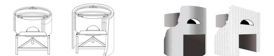
Once insulated, build the external masonry wall and finish the oven giving the aesthetic touch Oven mod. MEC 80 must be insulated and covered with fire resistant materials. Failure to follow the installation instructions could cause damages as fires.
